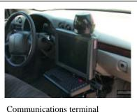
Communications terminal mounted in the deployment path of a passenger side frontal air bag. *Note the frontal warning device mounted to the screen*
