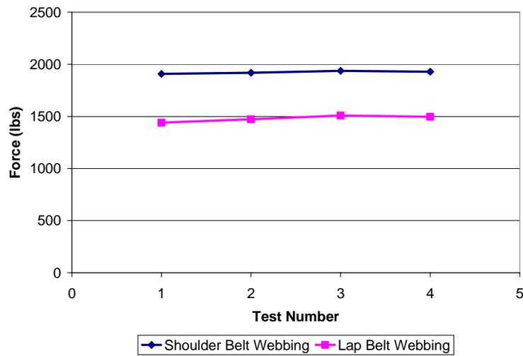
**Figure A 4. Mean force values for shoulder and lap belt webbing RAM for all four tests**
