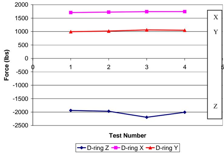
**Figure A 3. Mean force values for shoulder and lap belt RAM for all four tests**
