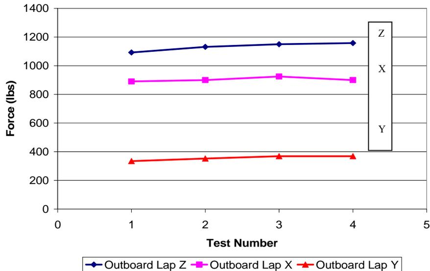
**Figure 3.** Mean force values for the outboard lap belt for all four tests
