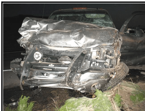
Figure 9. 2007 GMC C3500 front plane damage (police photo)
