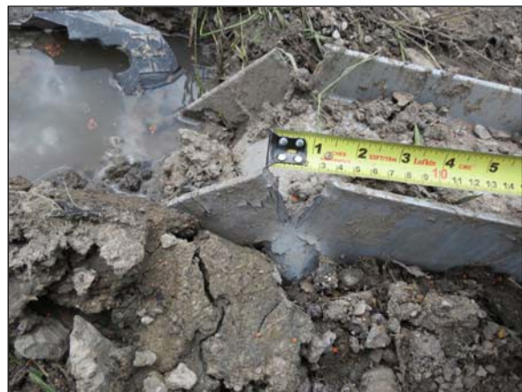
Figure 8: Crimp at base of Post 3
