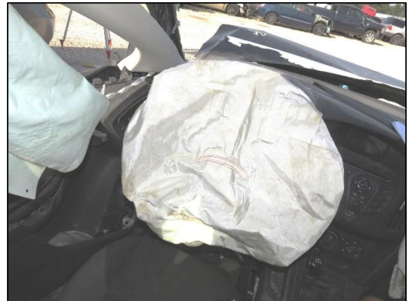
Figure 7: The Ford's driver's deployed frontal air bag, left IC, and left A-pillar
