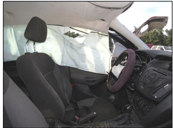
Figure 8: The Ford's deflated left IC air bag
