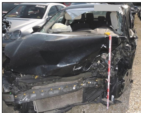
Figure 5: Damage to the front plane of the Ford from the impact with the Pontiac
