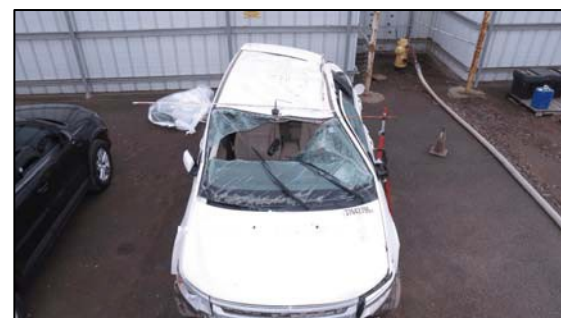
Figure 9. Top damage, 2013 Ford Edge
