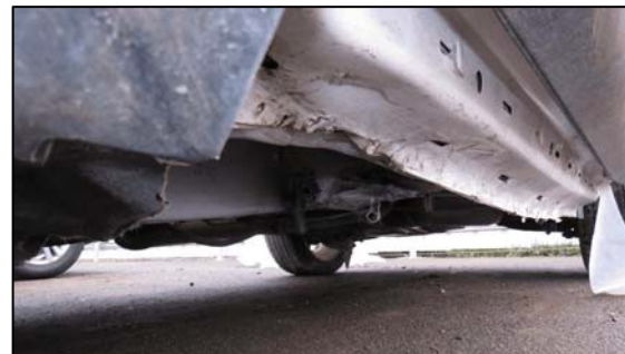
Figure 8. Left frame rail damage, 2013 Ford Edge
