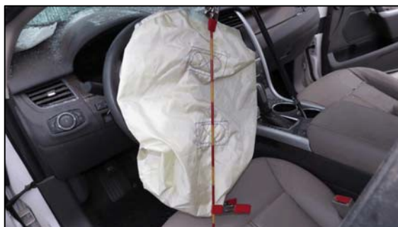
Figure 11. Driver's air bag, 2013 Ford Edge
