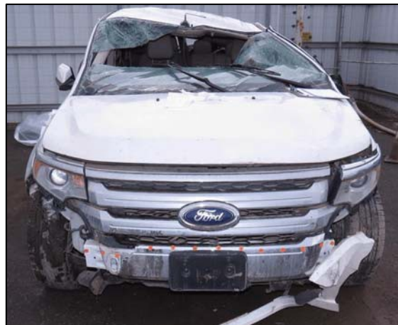
Figure 7. Frontal damage, 2013 Ford Edge
