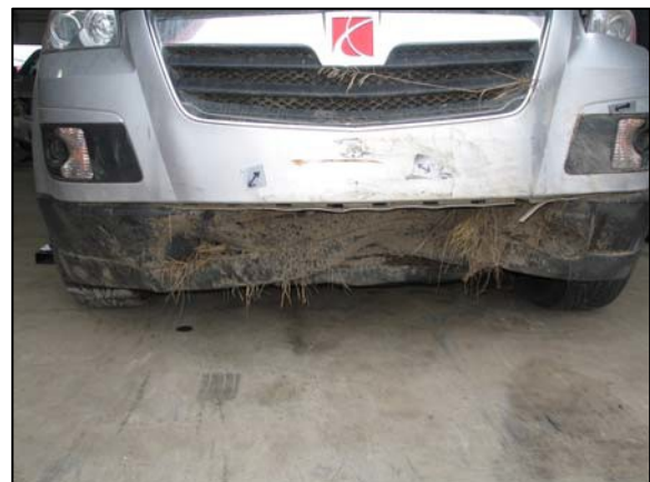
Figure 4: Front bumper fascia/undercarriage damage
