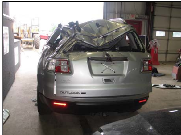
Figure 5: Maximum vertical crush at left D-pillar
