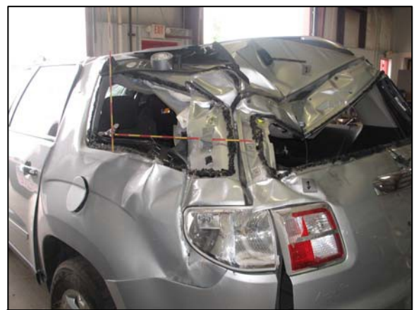
Figure 6: Maximum vertical crush
