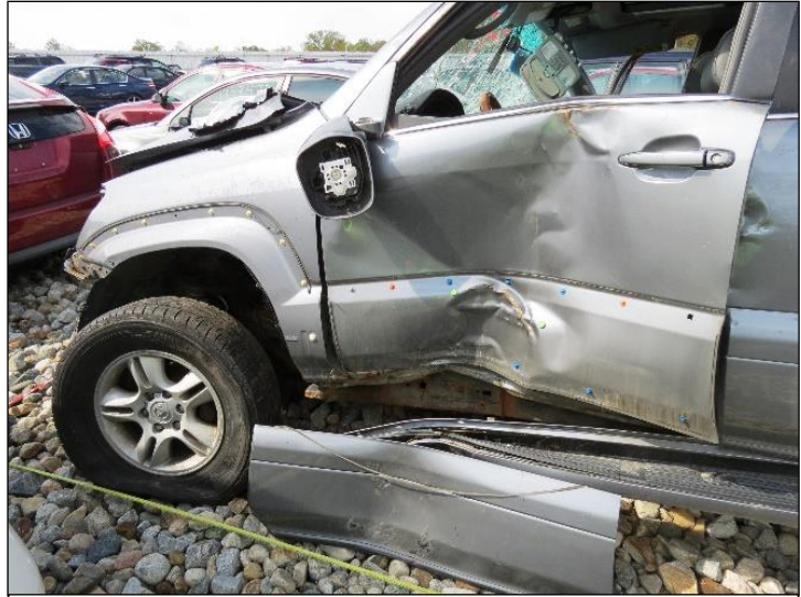
Figure 9: View of the left plane damage pattern to the Lexus from the Event 4 tree impact.
