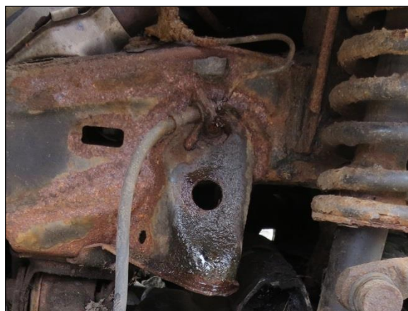
Figure 13: View of the corroded connection and leaking brake fluid during the SCI brake system test.
