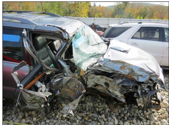
Figure 7: Damage pattern to the forward half of the Lexus' right plane.
