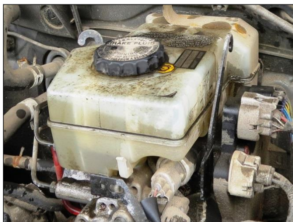
Figure 12: View of the layered brake fluids (dark – old, light – new) following refill of the reservoir by the SCI investigator.
