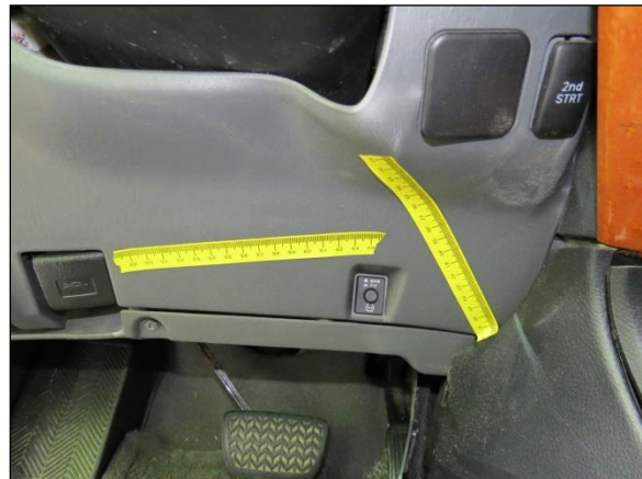
Figure 10: Deformation and scuffing on the left lower instrument panel from loading by the driver's knees.
