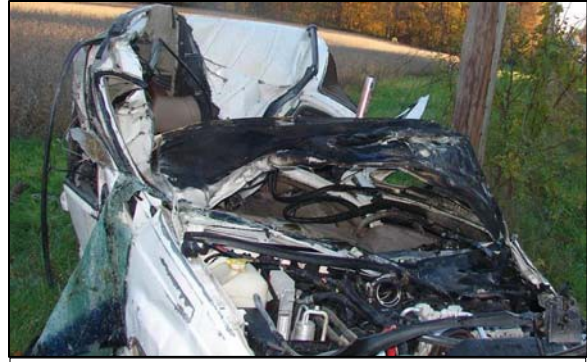
Figure 9: Area of fire damage to the Jeep
