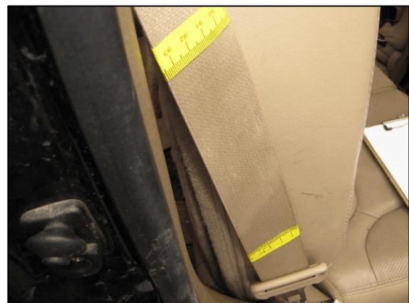
Figure 6. Second row right seat belt, evidence of occupant loading, 2006 Nissan Pathfinder
