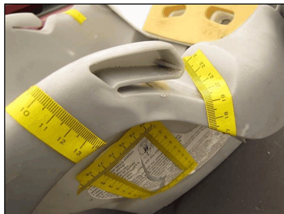
Figure 10. Occupant loading damage at rear-facing seat belt hook
