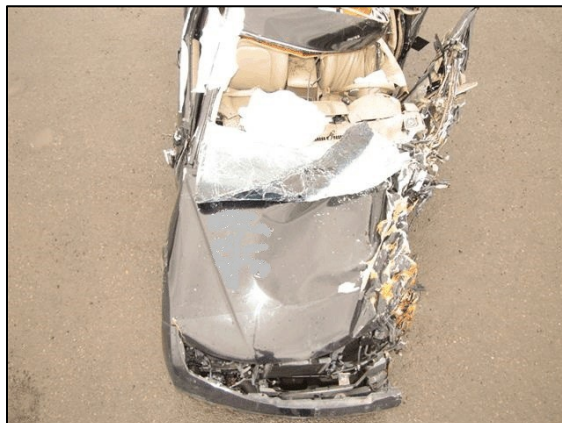
Figure 4. Exterior damage, 2006 Nissan Pathfinder
