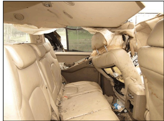
Figure 5. Vertical intrusion of roof, 2006 Nissan Pathfinder
