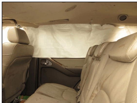
Figure 7. Deployed right IC air bag, second row right seat position, 2006 Nissan Pathfinder
