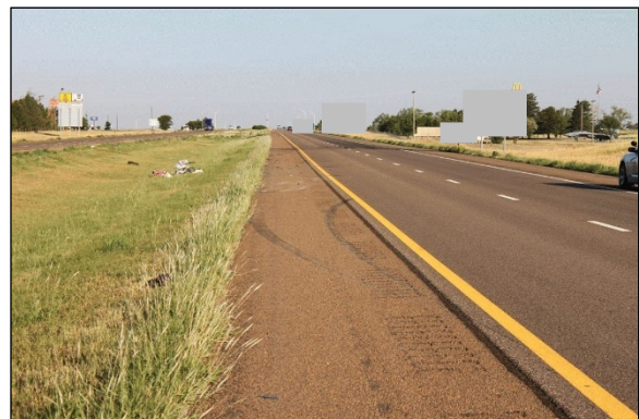
Figure 4: Police photo of Chevrolet's tire marks from driver's right steering maneuver and path to rollover, view northwest
