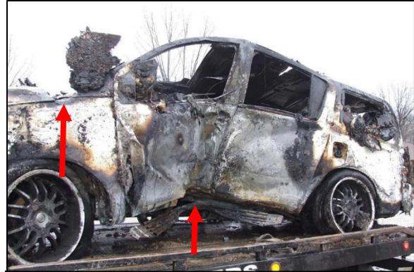
Figure 3: Police photo showing damage to top plane from post impact (left arrow) and damage to left plane from tree impact (right arrow)
