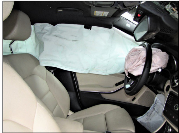
Figure 8. Deployed left IC air bag, 2017 Mercedes-Benz GLA 250
