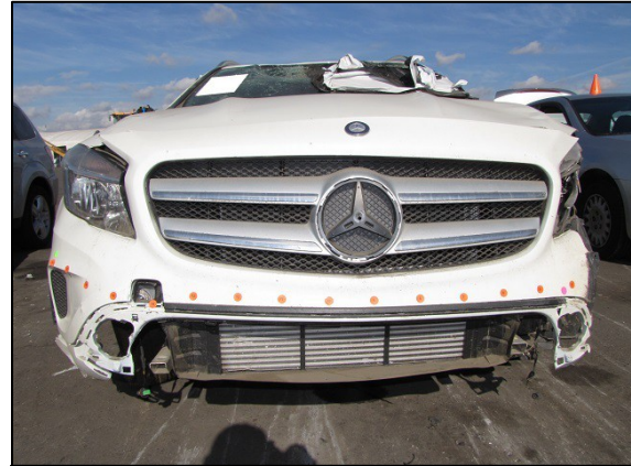
Figure 4. Front end crush measurements, 2017 Mercedes-Benz GLA 250
