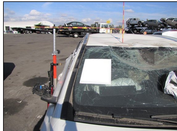
Figure 5. Rollover measurements, 2017 Mercedes-Benz GLA 250
