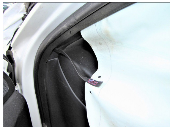
Figure 6. IC air bag tethered at bottom edge of side glass, 2017 Mercedes-Benz GLA 250
