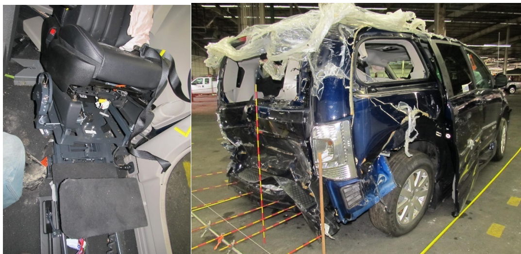
Figure 30: Case No. 20014-81-033 Post-Crash Damage to Seat Base and Vehicle
