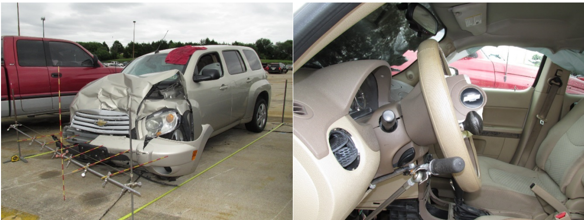
Figure 48: Case No. 2015-49-053 Chevrolet HHR Damage and Adaptive Equipment
