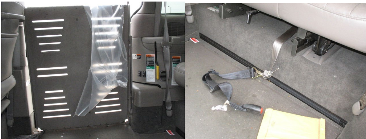
Figure 19: Case No. 2008-72-083 Wheelchair Ramp and Second Row Tie-downs
