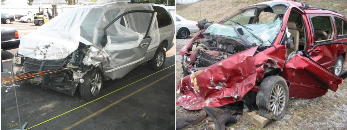
Figure 56: Case Nos. 2007-79-127 and 2009-45-021 and 51 and 62 km/h Delta-V Frontal Impact Respectively
