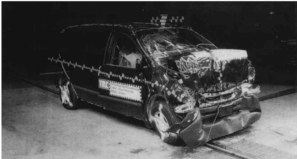
Figure 57: NHTSA Test No. 2997 1999 Dodge Caravan 56 km/h Frontal Crash Test
