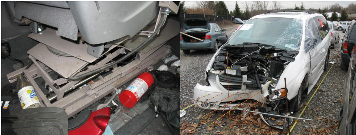
Figure 31: Case No. 2008-02-148 Post Crash Damage to Seat Base and Vehicle
