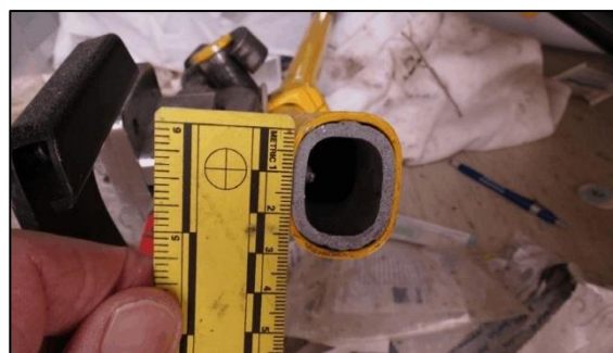
Figure 12. Lower frame rail damage at rail.
