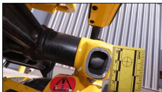
Figure 11. Lower frame rail damage at rear.
