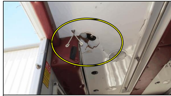
Figure 15. Contact evidence, probable injury source for patient, 2004 Ford E-350.
