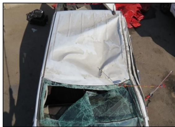
Figure 4. 2017 Ram 1500, top damage.
