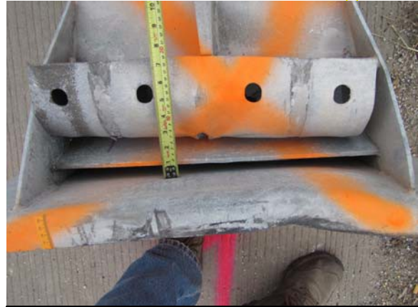
Figure 8. Extruded guardrail on field side of end terminal.
