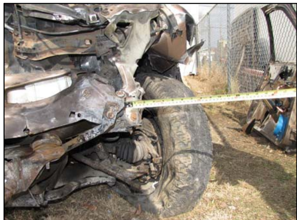
Figure 4. Area of end terminal impact.
