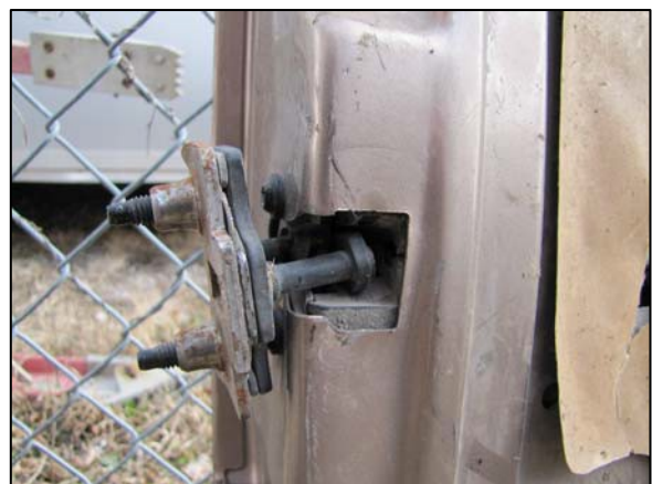
Figure 12. Striker remained in left front door latch.
