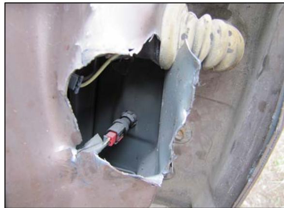
Figure 11. Chevrolet's torn door frame sheet metal where left front door striker was mounted.
