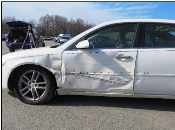
Figure 10. View of the Event #1 damage pattern to the 2009 Chevrolet Impala.
