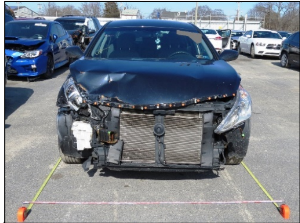
Figure 6. View of the front plane damage profile to the 2011 Hyundai Sonata.
