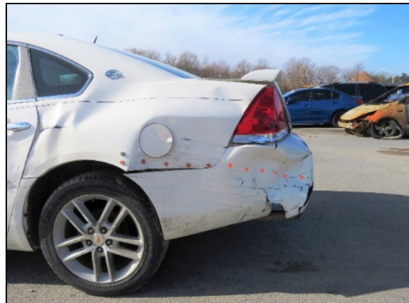
Figure 12. View of the Event #3 damage pattern to the 2009 Chevrolet Impala.
