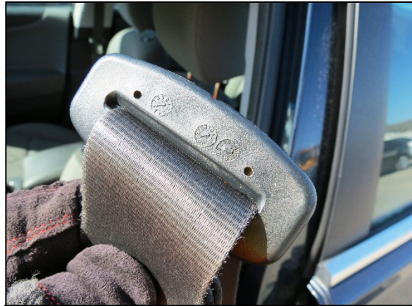
Figure 8. Latch plate of the Hyundai driver's seat belt system with minor loading abrasion evidence.
