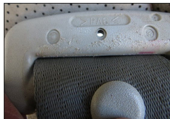
Figure 6. Right passenger seat belt latch loading, 2009 Lexus ES350.
