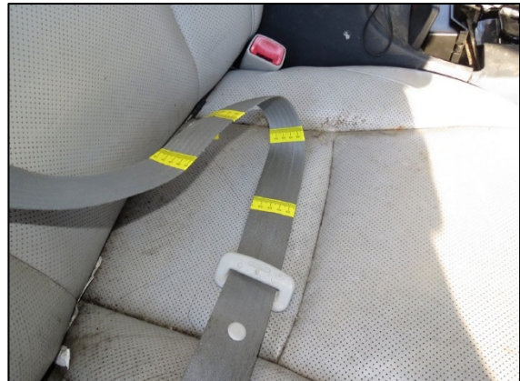
Figure 7. Right passenger lap and shoulder seat belt loading, 2009 Lexus ES350.
