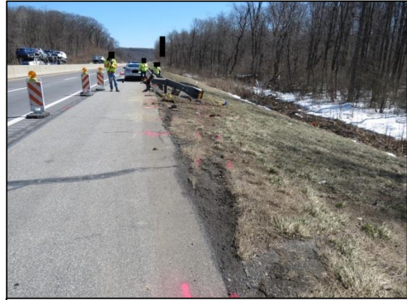
Figure 4. Easterly view of the left side tire yaw marks on the grass roadside.
