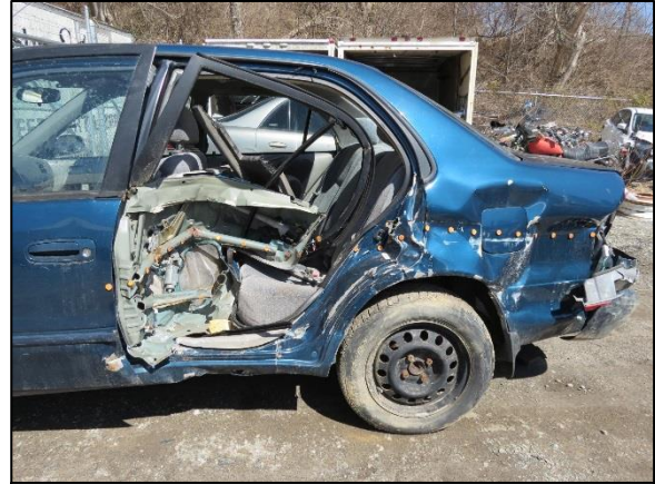
Figure 11. Left side view of the Toyota depicting the damage pattern.
