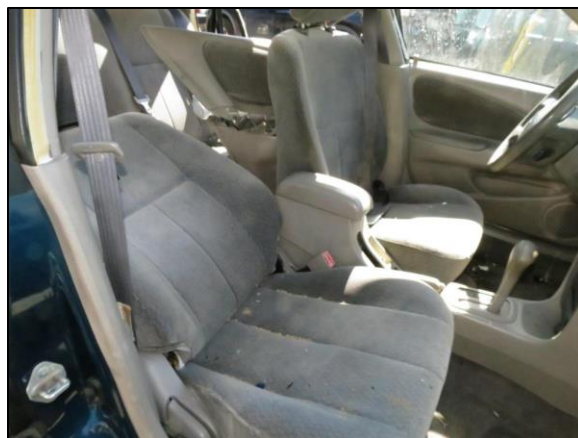
Figure 12. Overall interior view of the Toyota and the rearward deflection of the front row right seat back.
