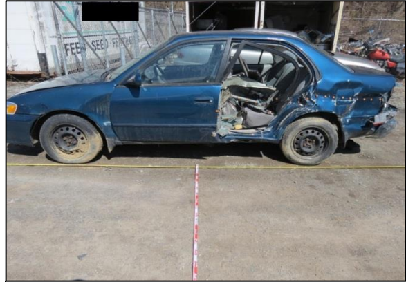
Figure 10. Left plane damage to the Toyota.
