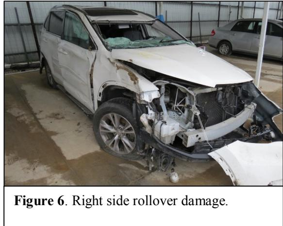
**Figure 6.** Right side rollover damage.
