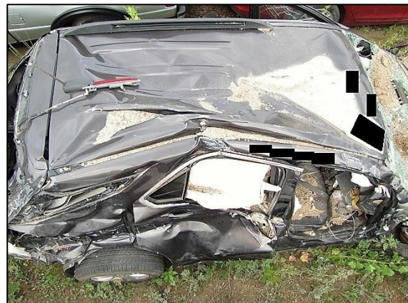
Figure 6. 2016 Chevrolet Equinox right plane damage.
