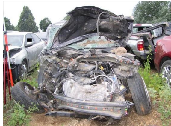
Figure 5. 2016 Chevrolet Equinox front plane damage.
