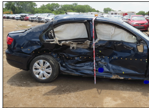
Figure 4: Damage to the Volkswagen's right plane from impact by the front plane of the Chevrolet
