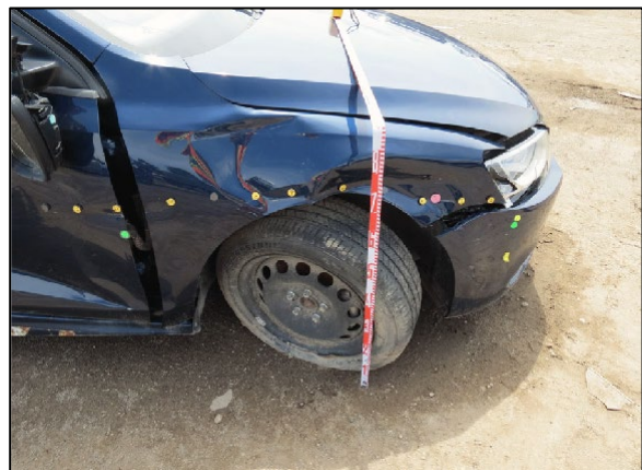
Figure 5: Damage to the Volkswagen's right fender from impact with the Chevrolet's right fender
