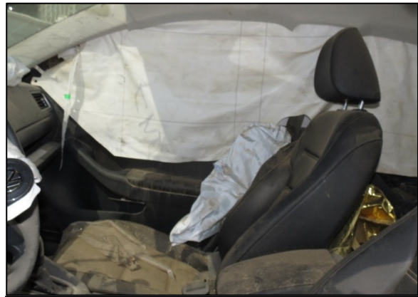
Figure 7: The Volkswagen's deflated front right seat-mounted side impact and right IC air bag
