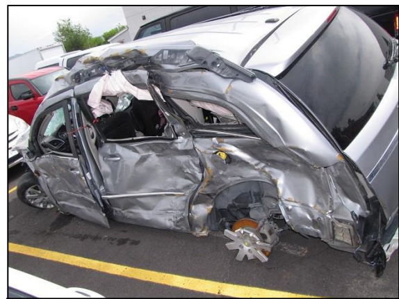
Figure 3. Left plane damage, the 2016 Chrysler Town & Country.
