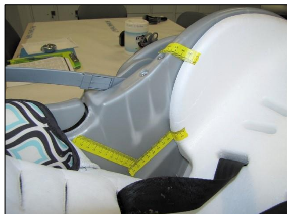
Figure 6. Baby Trend Flex-Loc damage to shell, the 2016 Chrysler Town & Country.
