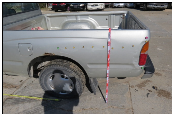
Figure 4. Sideswipe damage to the left side of the Toyota's truck bed.
