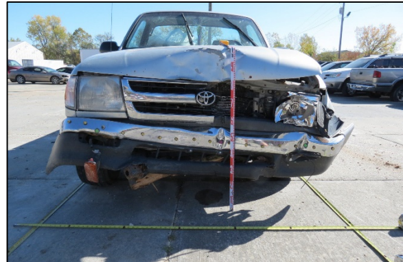
Figure 6. Damage to the front plane of the Toyota from the impact with the end terminal.
