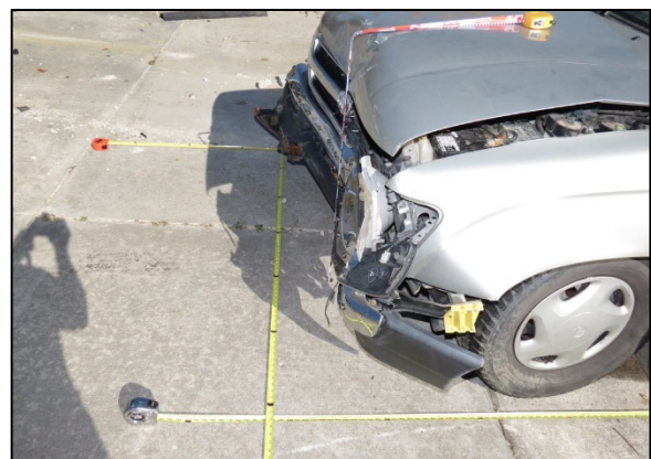
Figure 8. Left lateral view depicting the crush of the Toyota.
