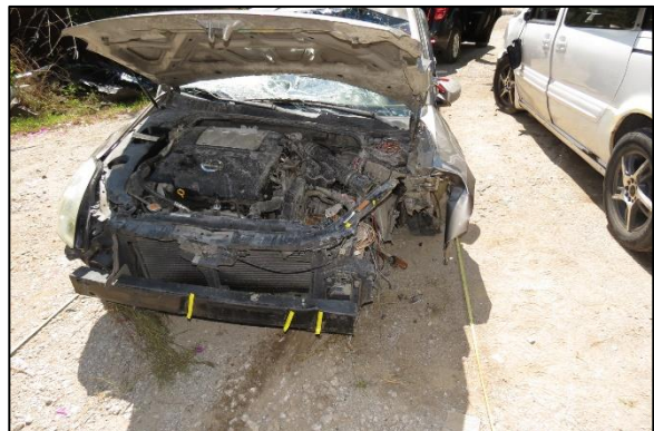
Figure 10. Front view of the Nissan depicting the damage of Events 1 to 3.
