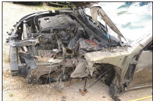
Figure 5. Damage to the Nissan from the impact with the end terminal.
