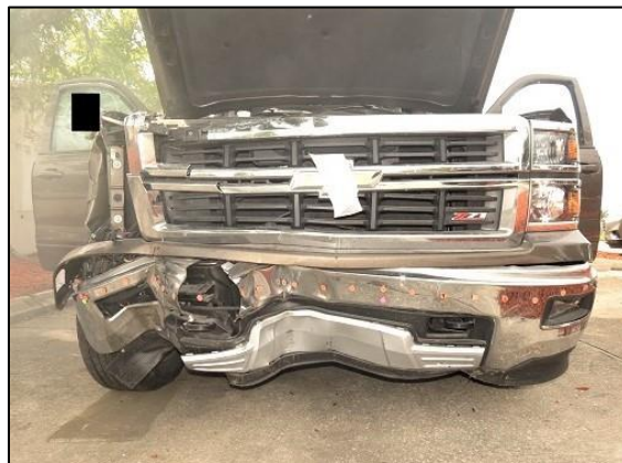
Figure 4. Front-plane damage, the 2015 Chevrolet Silverado.
