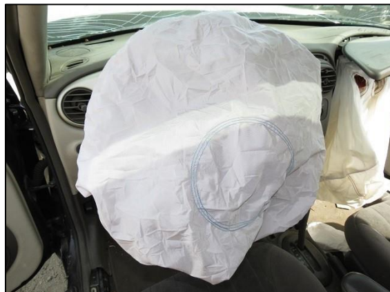
Figure 6. Driver's deployed front air bag, the 2002 Chrysler PT Cruiser.
