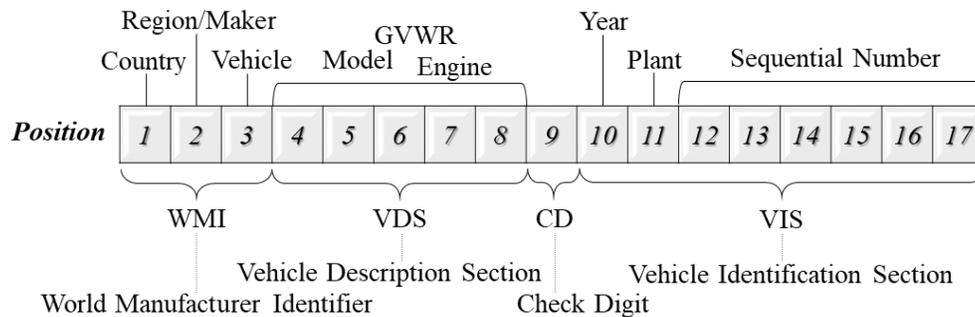
*Figure 4. Components of 17-Digit Full Vehicle Identification Number.*
