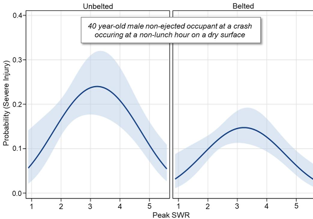
*Figure C1. Predicted probabilities for a 40-year-old male non-ejected occupant sustaining a severe injury in a rollover crash occurring at a non-lunch hour on a dry surface by peak SWR based on the polynomial binary logit model.*
