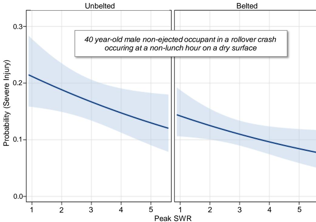
Figure 13. Predicted probabilities for a 40 year-old male non-ejected occupant sustaining a severe injury in a rollover crash occurring at a non-lunch hour on a dry surface by peak SWR. A solid line corresponds to a predicted probability in a varying condition and a shade area encompassing the line corresponds to 95 percent Wald-test-based confidence limit. A severe injury includes a fatal or incapacitating injury.
