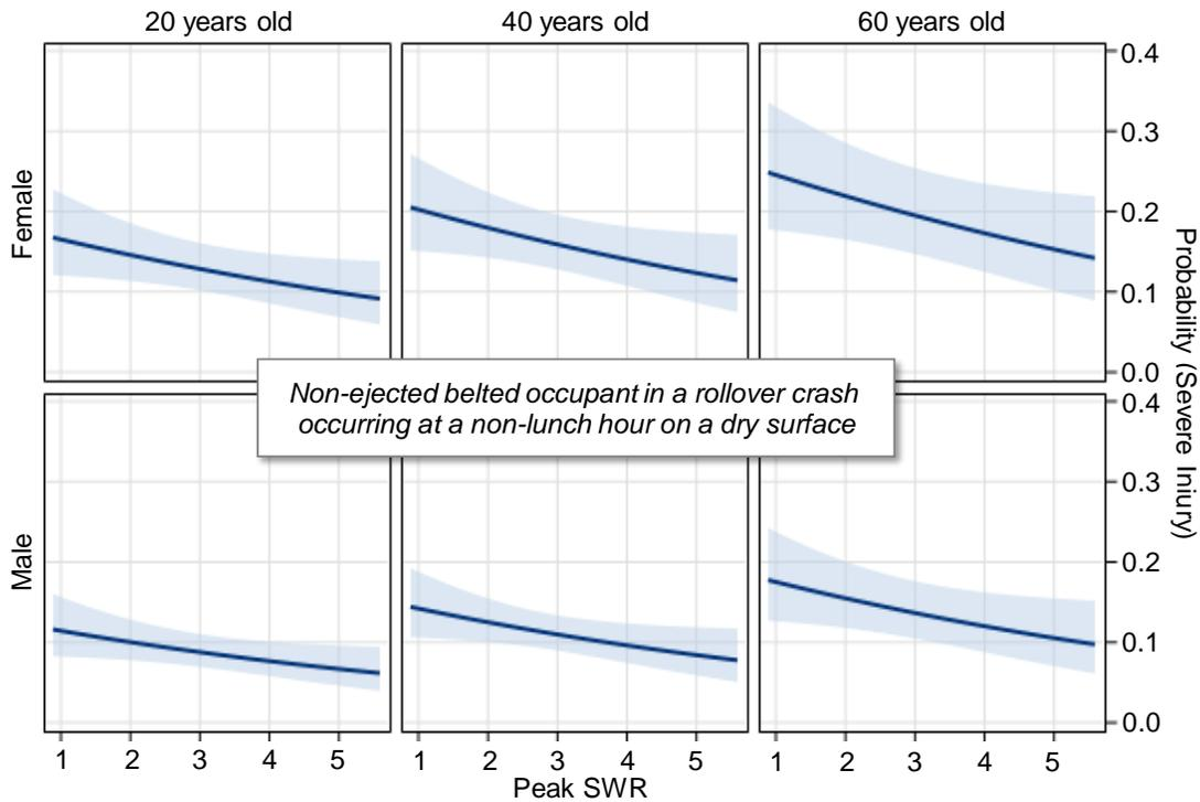
Figure 14. Predicted probabilities for a non-ejected belted occupant sustaining a severe injury in a rollover crash occurring at a non-lunch hour on a dry surface by peak SWR. A solid line corresponds to a predicted probability in a varying condition and a shade area encompassing the line corresponds to 95 percent Wald-test-based confidence limit. A severe injury includes a fatal or incapacitating injury.
