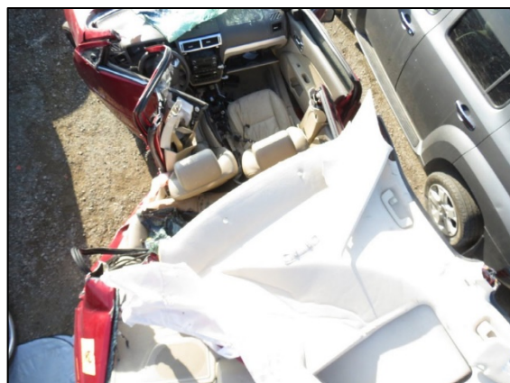
Figure 7. Interior damage, the 2008 Mercury Milan.
