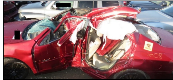
Figure 6. Left plane damage, the 2008 Mercury Milan.
