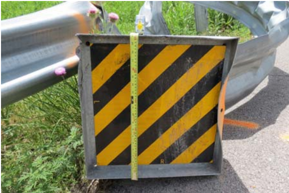
Figure 5. Southerly view, impact face. (Note - vertical tire tread)
