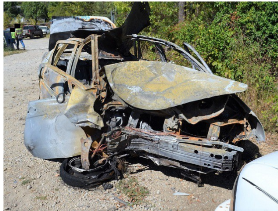
Figure 3. Front plane damage, 2009 Ford Focus (police photo)
