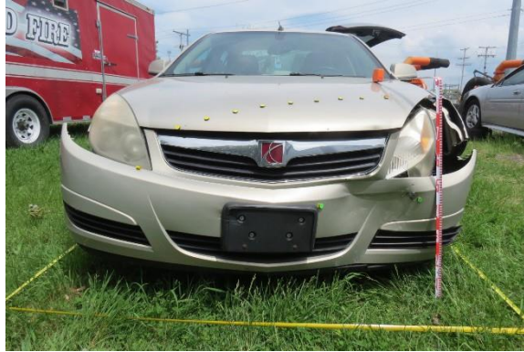
Figure 6. Front plane damage to the Saturn
