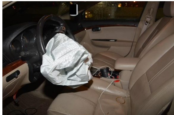
Figure 8. On-scene police image of the Saturn's interior. The steering wheel is rotated an estimated 30 degrees to the left (counter-clockwise)
