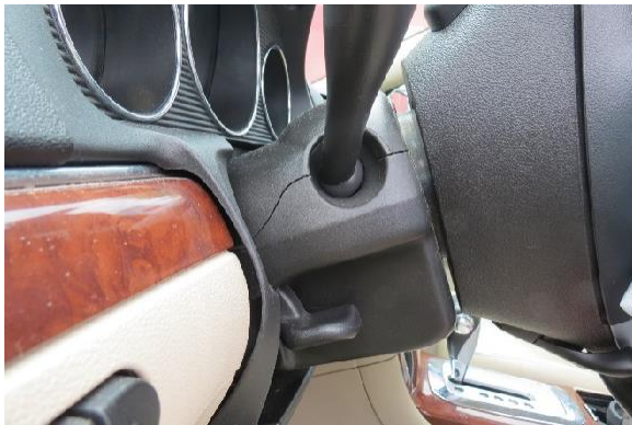
Figure 7. Disparity in gap between Saturn's steering wheel hub and column. Note: wheel was rotated 90 degrees to the left at the time of the SCI inspection
