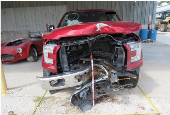
Figure 7. Frontal damage from the Event 2 tree impact with dirt embedded from the Event 1 impact
