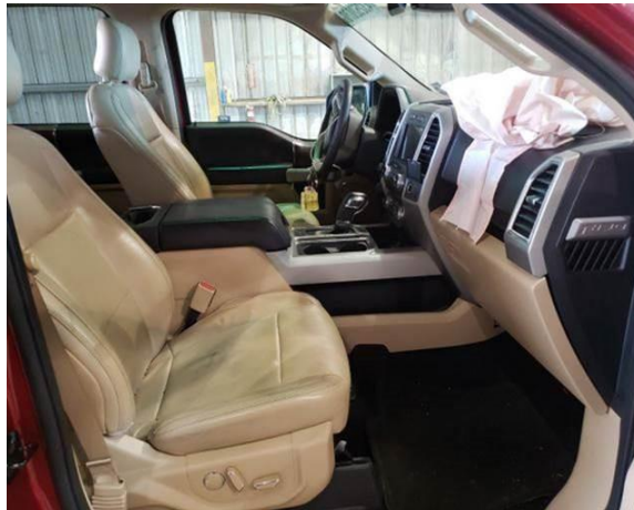
Figure 1. View of the deployed passenger's frontal air bag in the 2017 Ford F-150 (image provided by the salvage facility)
