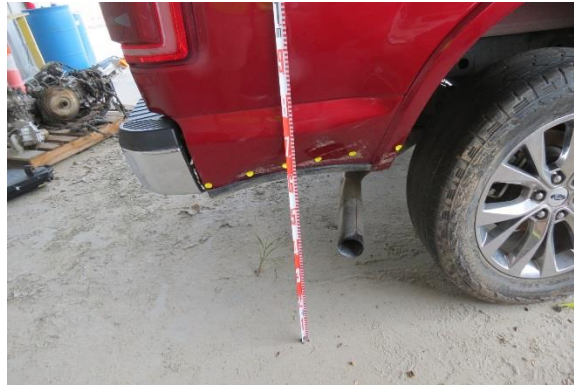
Figure 9. Event 3 damage to the lower right aspect of the cargo box
