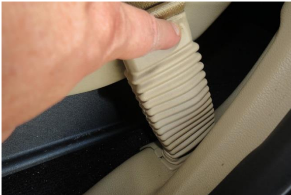
Figure 10. Actuated driver's lower anchor pretensioner
