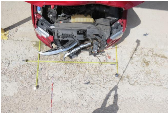
Figure 8. Overhead view showing the extent of frontal crush
