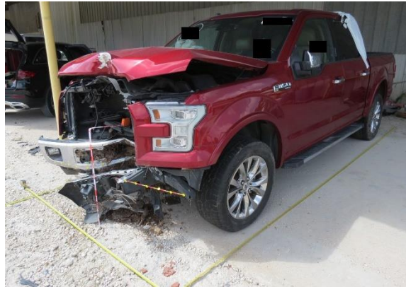
Figure 6. Frontal damage from the Event 2 tree impact with dirt embedded from the Event 1 impact
