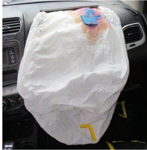
Figure 9. View of the deployed right front passenger's frontal top instrument panel air bag
