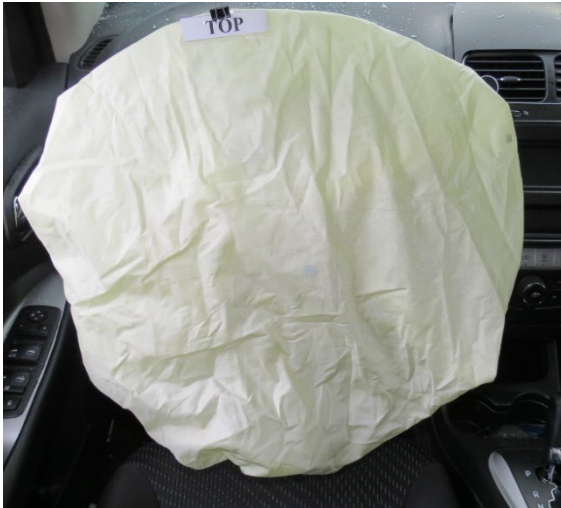
Figure 8. View of the deployed driver's frontal steering wheel hub-mounted air bag
