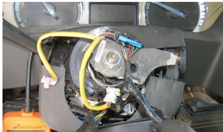
Figure 18. Close-up image showing the two wire leads from the clockspring and the undamaged squib connectors
