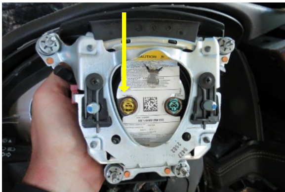
Figure 14. Backside of the driver's frontal air bag module and the inflator
