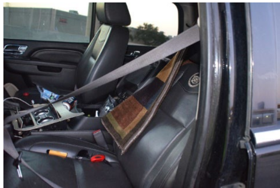
Figure 12. On-scene police image documenting the intact driver's seat belt system prior to being cut for unknown reasons
