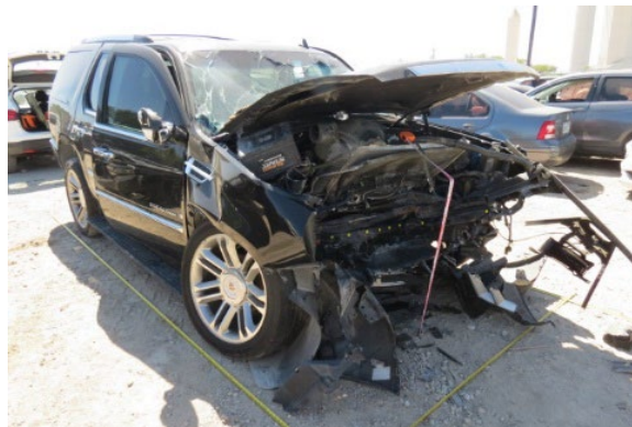
Figure 7. Front right oblique view showing the severity of the frontal damage
