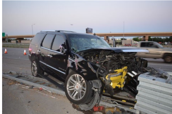
Figure 6. Northeast view, on-scene police image of the Cadillac engaged with the compressed impact attenuator
