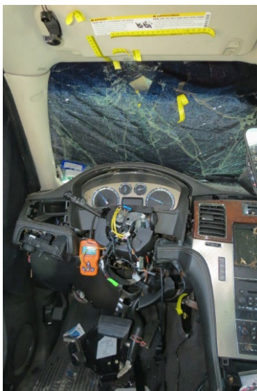
Figure 11. Overall image of the left forward interior showing the driver contacts
