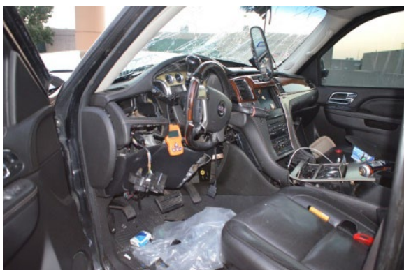
Figure 9. Overall view of the driver's compartment and the occupant contact to the frontal components (image provided by the investigating police officer)
