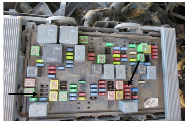
Figure 16. Image showing the underhood fuse panel of the Cadillac
