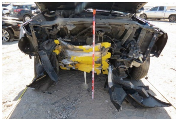
Figure 8. Frontal damage to the Cadillac with the face of the attenuator still engaged in the damage
