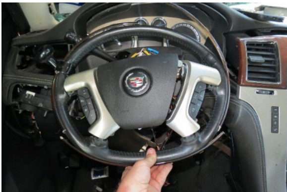
Figure 13. Driver's frontal air bag module in the fractured hub/spokes of the steering wheel
