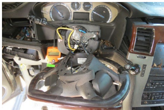
Figure 10. SCI inspection image of the observed position of the fractured steering wheel rim and wiring
