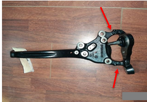
Figure 10. Exemplar Dodge Challenger right front suspension knuckle
