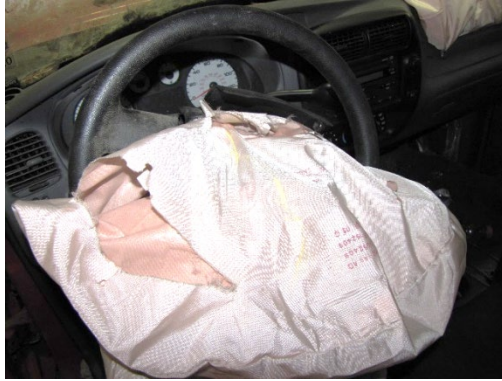
Figure 10. View of the tear in the fabric on the back side of the driver's frontal air bag in the Ford
