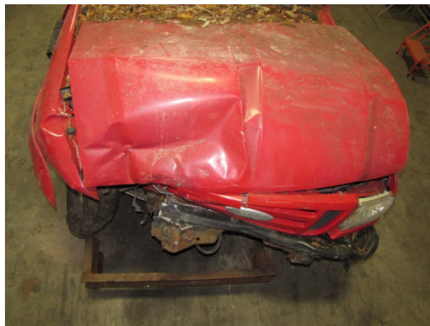
Figure 6. Overhead view of the crush profile to the Ford
