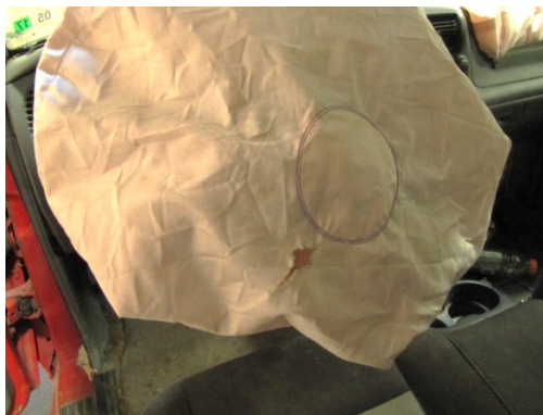
Figure 9. Overall view of the tear in the face of the deployed driver's frontal air bag prior to removal from the Ford
