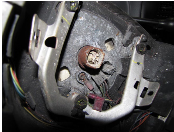
Figure 13. Close-up image of the center aspect of the Ford's steering wheel and the driver's frontal air bag squib separated during the deployment
