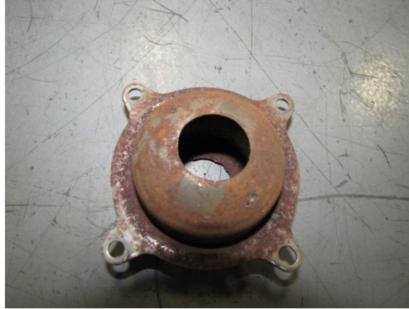
Figure 15. Front aspect of the inflator depicting the separated top area of the Ford's inflator. The separated (missing) fragment penetrated the air bag fabric and struck the driver's chest.
