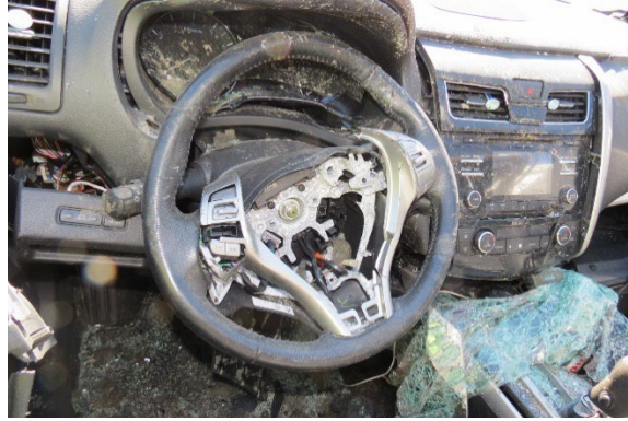
Figure 11. View of the Nissan's deformed steering wheel
