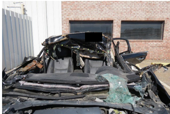
Figure 9. Underride direct damage from impact to the back of the trailer
