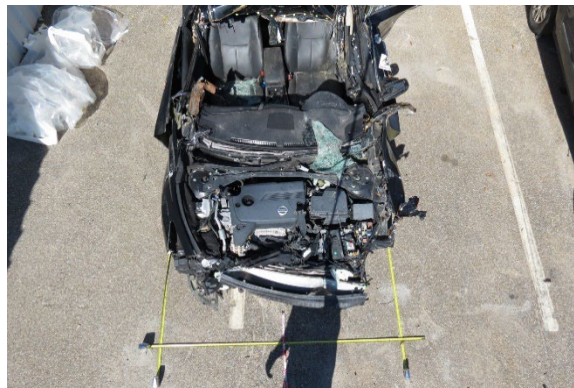
Figure 6. Overhead view of the Nissan depicting the frontal underride damage
