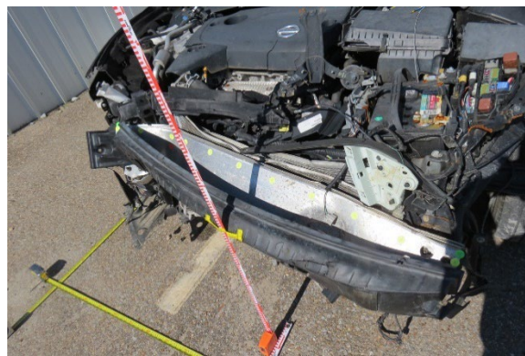
Figure 8. Frontal plane direct contact damage from impact to the back of the trailer
