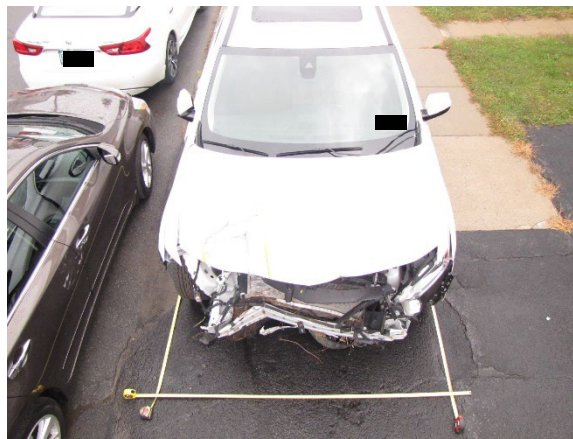
Figure 4. Overhead view of the Chevrolet depicting the frontal deformation
