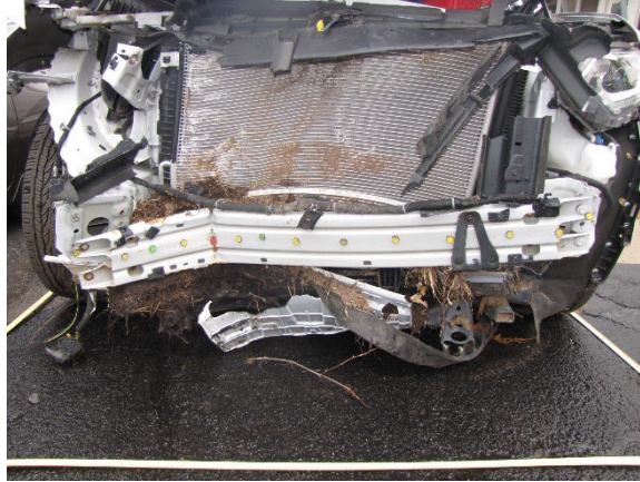
Figure 5. Close-up view of the Chevrolet's frontal deformation
