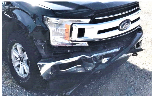
Figure 3. View of the Ford's front-plane damage pattern (repair facility provided image)
