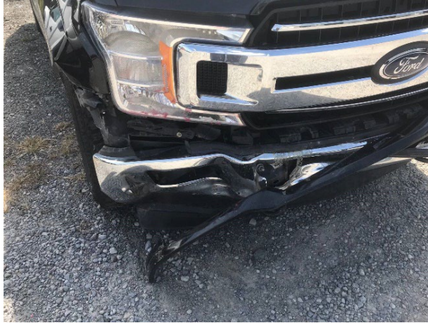
Figure 4. Close-up view of the Ford's front-plane damage pattern (repair facility provided image)
