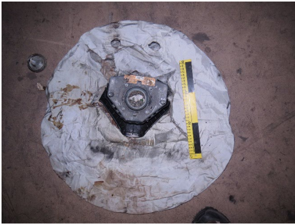
Figure 11. Back of air bag, air bag module, 2002 Volvo S60
