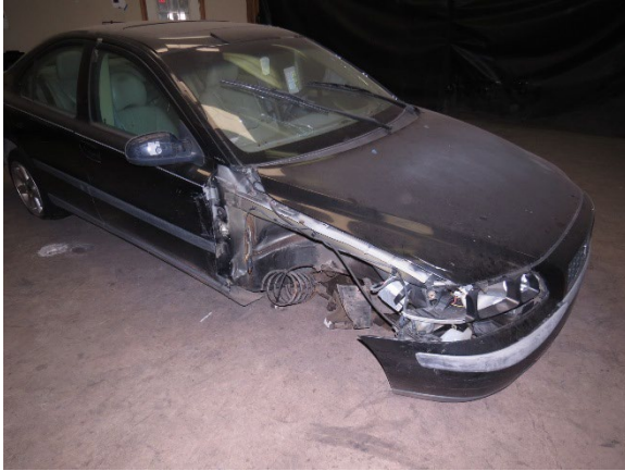
Figure 5. Front/right damage, 2002 Volvo S60
