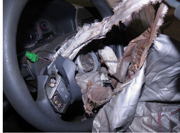
Figure 8. Driver frontal air bag inflator, attached to the vehicle, 2002 Volvo S60
