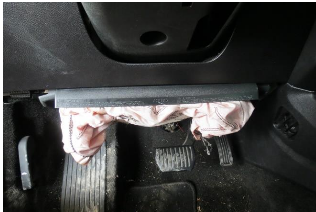
Figure 11. Packed knee air bag with upper flap opened
