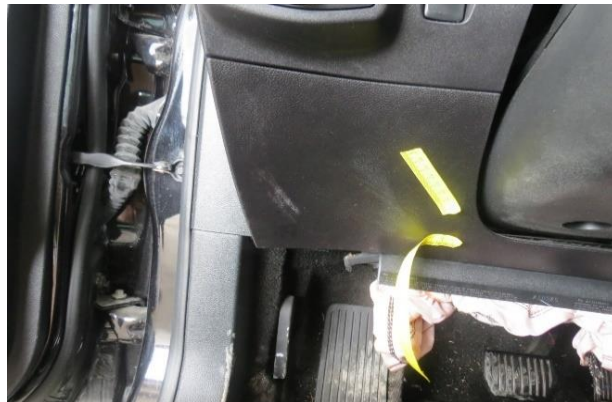
Figure 9. Left knee bolster contact
