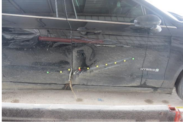
Figure 5. Sideswipe damage to the Ford's right doors
