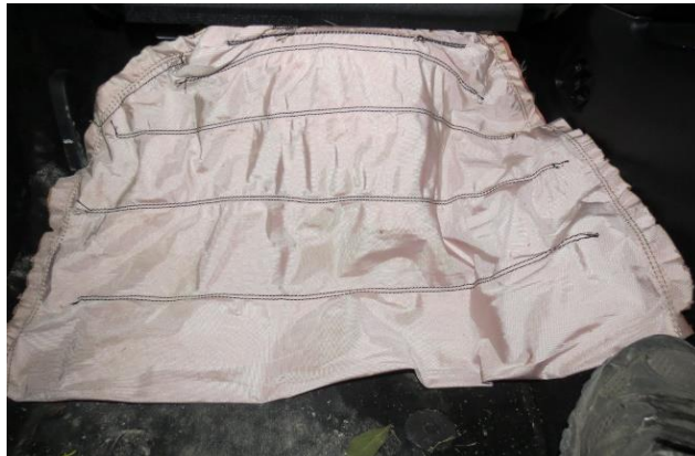
Figure 10. Deployed knee air bag
