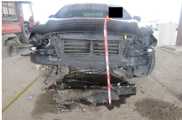
Figure 6. Front end damage to the Ford. Note bottom stabilizer bar.
