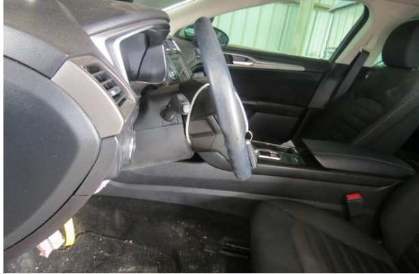
Figure 7. Steering wheel rim of the Ford bent slightly forward
