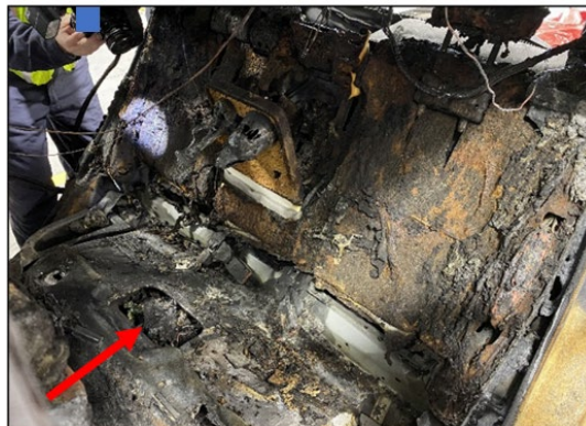
Figure 8. Service disconnect in the second row of the 2019 Chevrolet Bolt after the bottom seat cushion was removed
