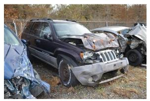
Figure 4. Front right oblique view of the frontal damage to the 2004 Jeep Grand Cherokee
