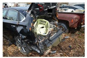
Figure 5. Back damage to the Nissan Altima following the Event 5 crash with the Jeep
