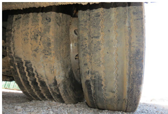
Figure 5. 4 mm (5/32 in) tread on left rear tires
