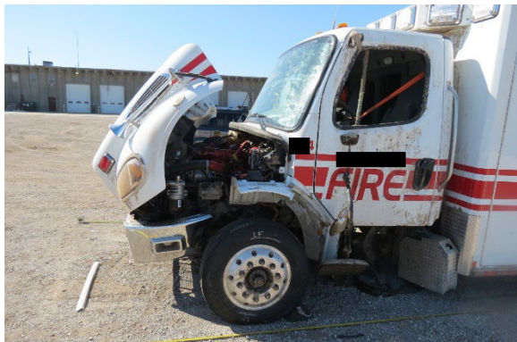
Figure 6. Ambulance cab rollover damage
