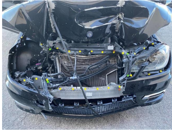
Figure 4. Front plane damage to the Mercedes-Benz
