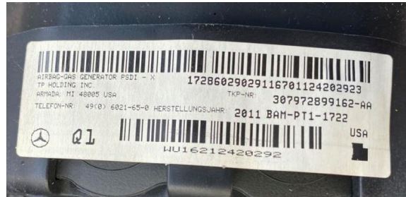
Figure 9. Driver's air bag module bar-coded label providing identification
