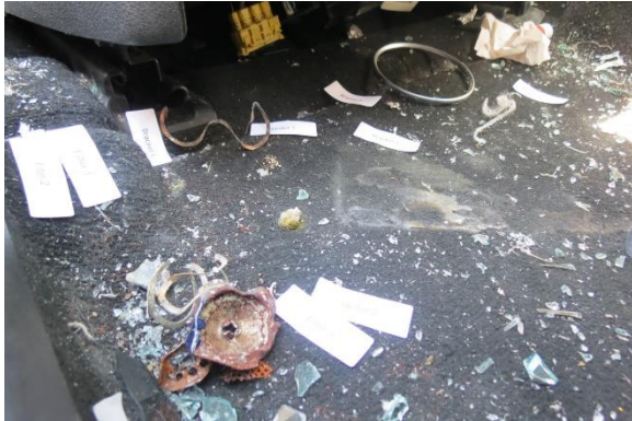
Figure 14. View of passenger floorboard showing air bag module components with labels as found
