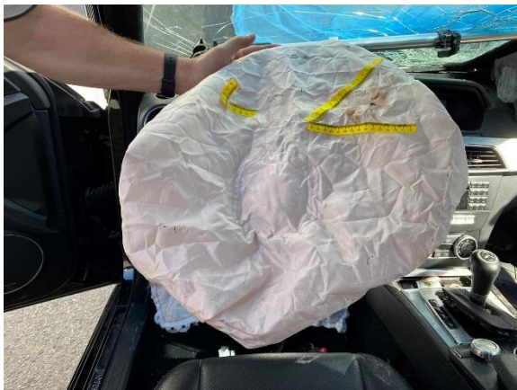
Figure 7. Deployed driver's frontal air bag and blood transfers of the upper right
