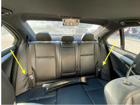
Figure 6. 2012 Mercedes-Benz second row pretensioner actuation evidence
