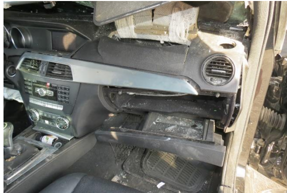
Figure 11. View of the front right instrument panel after removal of air bag and air bag module components during the SCI Inspection
