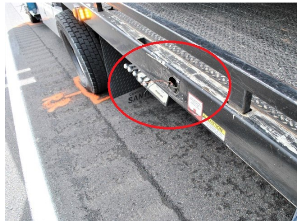
Figure 5. Left plane damage, 2018 Freightliner M2 (police photo)
