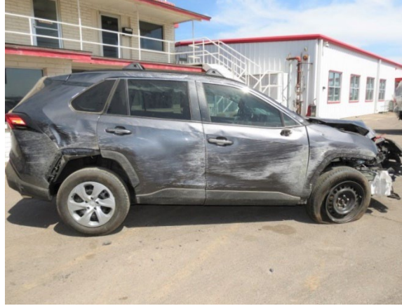
Figure 8. Right plane damage, 2021 Toyota RAV4
