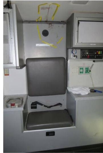
Figure 7. Contacts/blood stains on patient compartment, left side contact area/final rest
