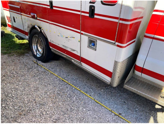
Figure 4. Right plane damage to Ford
