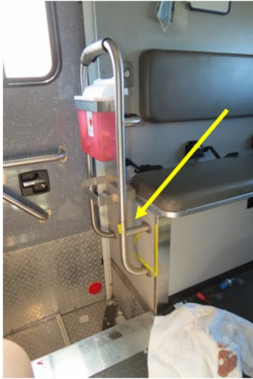
Figure 6. Railing contact on right side of patient compartment
